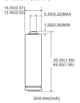
Chemical System: Alkaline (Zn/MnO<sub>2</sub>) Zinc-Manganese Dioxide
